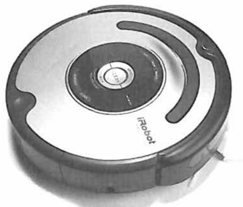
FIGURE AP1.6 A robotic vacuum cleaner communicates with the base station as it maneuvers around the room. (Photo courtesy of Alamy Images.)
